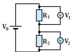
A potential divider is used to produce a desired potential difference, it can be thought of as a potential selector.
