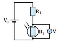
In the second potential divider the second resistor is a Light Dependant Resistor. When the light levels are low the resistance ( $R_2$ ) is high, making the output voltage high. When the light levels increase the resistance ( $R_2$ ) decreases, this makes the output voltage decrease. A use of this could be a street light sensor that switches the light on when the surroundings are dark.
