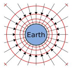
**Figure 2.** Equipotential lines surrounding a mass (shown as red concentric circles)
