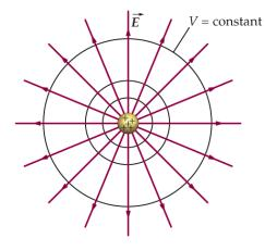
**Figure 1**. Equipotential lines surrounding a point charge (shown as black concentric circles)
